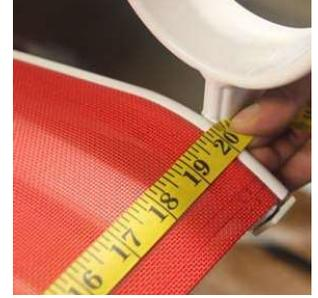
Starting a few inches down from the end of the metal sling rails, place your tape measure where the fabric disappears into the frame or rail and measure across to the other side. Measure up to the closest 1/4". Repeat for the bottom width.
