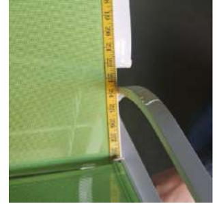
Starting a few inches down from the end of the rails, place your tape measure where the fabric disappears into the frame or rail and measure across to the other side. Measure up to the closest 1/4". Repeat for the bottom width. Starting at the top of the chaise back, measure the length of the back following the sling rail to the end.
