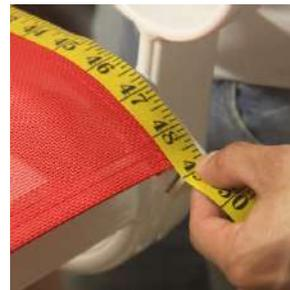
**DO NOT** measure the old sling. Measure on the chair frame with the old sling tightly installed. We will add the necessary fabric for hems and fabric inside the sling rail.
